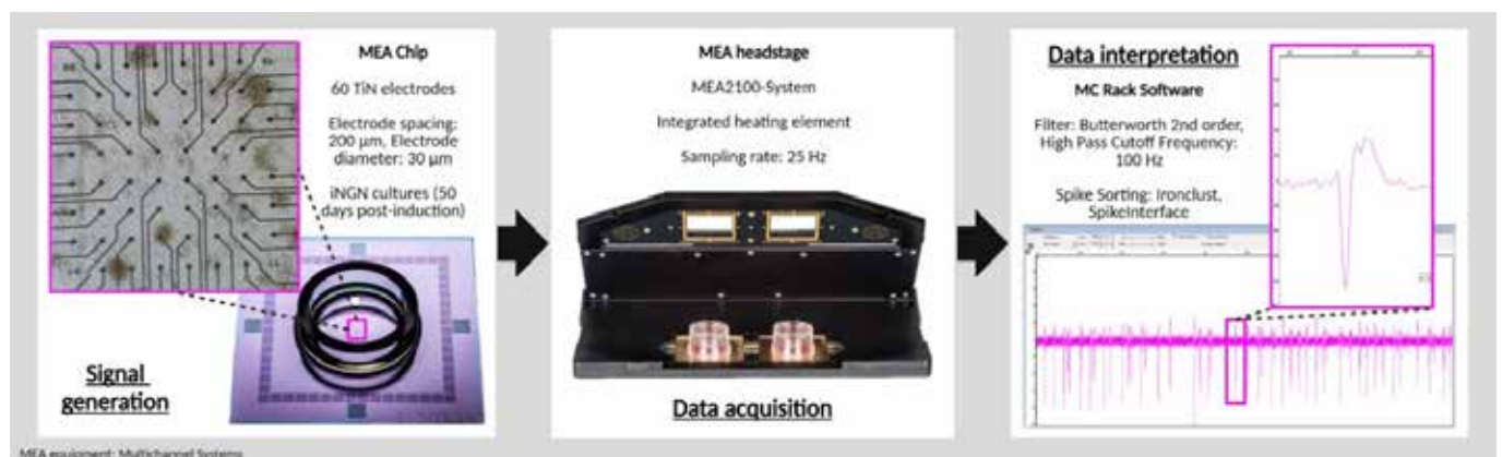
Fig. 1: MEA system workflow. TiN = titanium nitride, iNGN = inducible neurogenin cell line (Busskamp et al., 2014)
