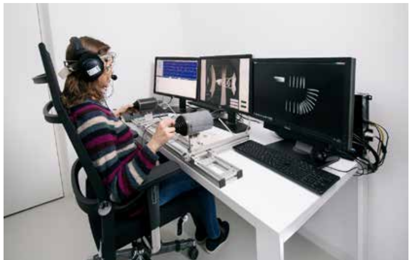
Fig. 3: Setup of the desktop-based 6df simulation. The left hand control is used for translational movements and the right one for rotational movements.
